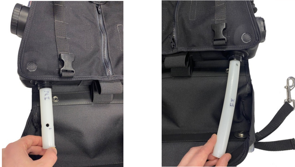
Figure 1 – Inserting Water Trap Tubes—Inhale on Left, Exhale on Right (note hole location)
