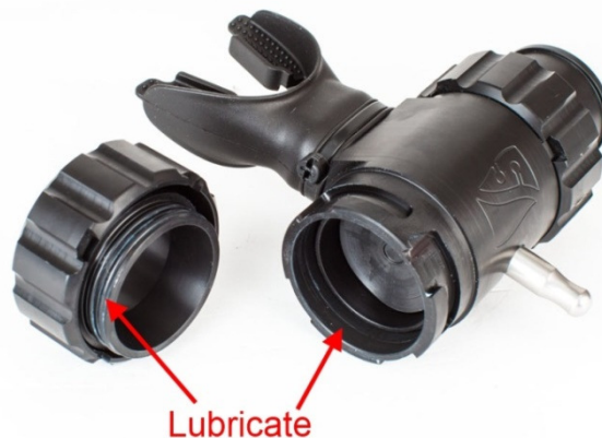
Figure 25 - Lubricate DSV Sealing Surfaces
