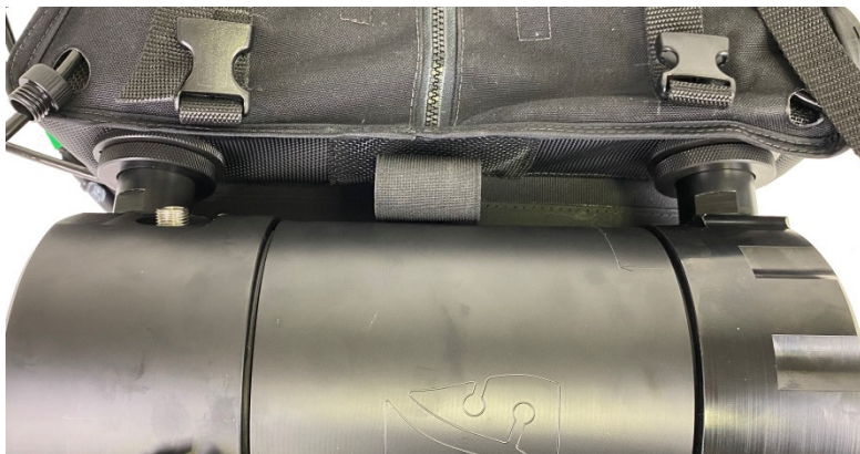
Figure 20 - Scrubber Canister Installed
