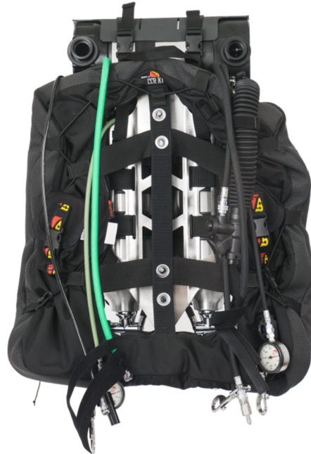
Figure 20 - Hose Routing Through Wing
