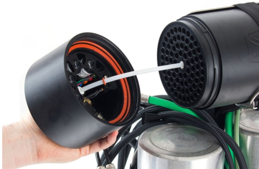
Figure 11 – Installing Electronics Head
